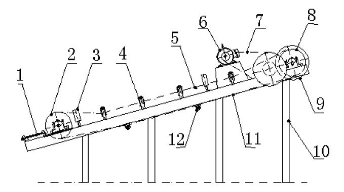
It mainly consists of 1 pulling device, 2 direction-changed roller, 3 belt-holding roller, 4 upper roller, 5 belt, 6 electric motor, 7v-belt, 8 transmission gear, 9 transmission roller, 10 supporting frame, 11 machine frame, and 12 lower roller as indicated in the following diagram.
