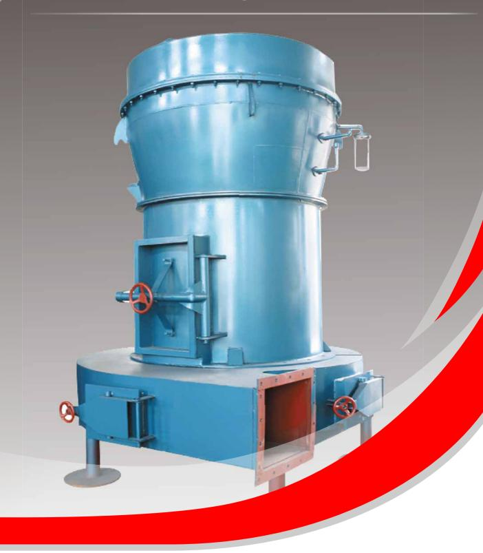
Raymond Mill is used to grind barite, calcite, potash feldspar, talcum, marble, limestone, ceram and slag below scale 7 of Moths hardness and 280-odd sorts of non-inflammable and non-explosive stuff in the traded of mining, building material, chemical engineering and metallurgy for power generation and processing. The product size is adjustable on required in the range of 100-325 meshes.
