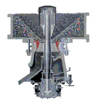
eccentric sleeve. When the eccentric sleeve rotates, there is a conical surface lined out by the shaft. When the movable cone comes near the fixed cone, rocks are grinded into pieces, when the movable cone leaves, grinded materials is discharged from the discharge hole. The fixed cone can be ascended or descended by adjusting setting to adjust the width of discharge hole, consequently the output size is determined adjusted.
