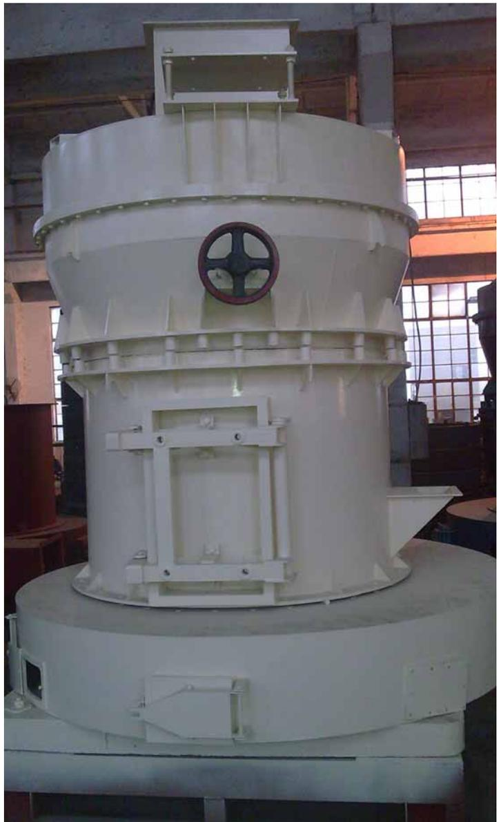
This mill consists of main frame, decelerator, powder separator, blower, jaw crusher, bucket-elevator, vibrating feeder, hopper ,bag filter, pipe—devices ,motor and electric switch box, etc..
